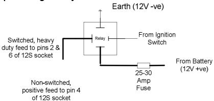
The purpose of the split charge relay is to prevent the caravan from flattening the battery of the towing vehicle.
